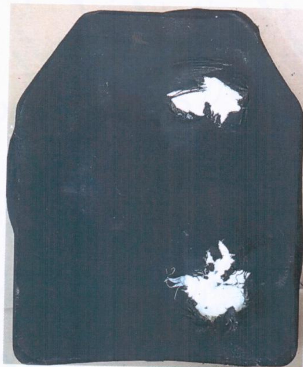
Fig. 2 Bullet Proof Plate 22032003(wear face)
