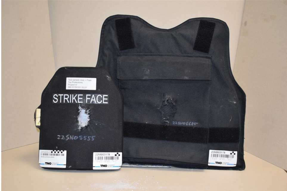
Strike Face, sample 22SA03573 after test 22MB03178
