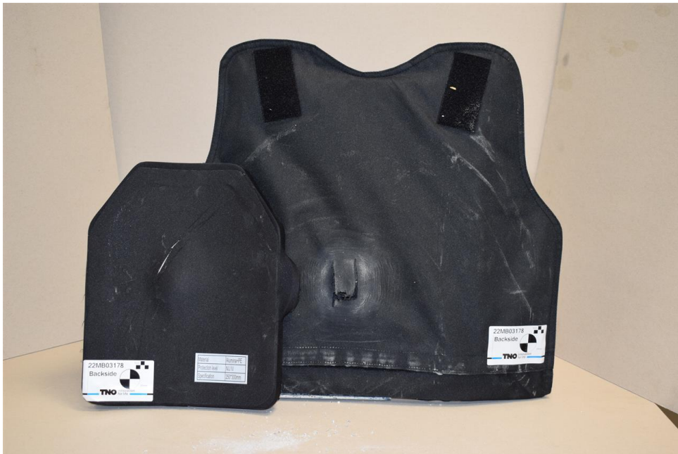
Back Face, sample 22SA03573 after test 22MB03178
